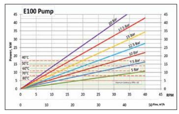
**Note:** Green area covers pump continuous operation. Pump can run at higher speed, which falls under intermittent regime, but requires periodical cooling.
